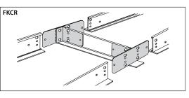
For flanged fixtures in row configurations, the FKCR adapter bracket kit is required in addition to the FK22 kit. Order one less FKCR than the total number of fixtures in row. (Example: Row of two, order (2) FK22 & (1) FKCR)
