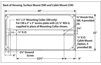
Order SM ceiling type. Mounting collar required for surface mounting.
