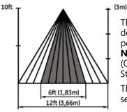
The detection area determination was performed according to the **NEMA WD 7-2011** Standard (Occupancy Motion Sensors Standard).
