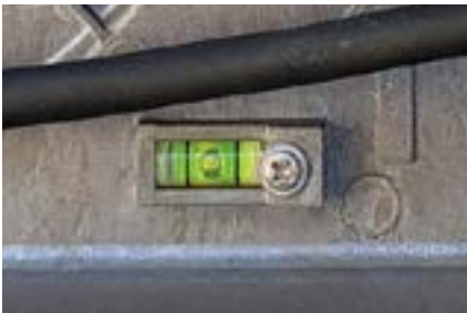
Incorporated level system in fixture
