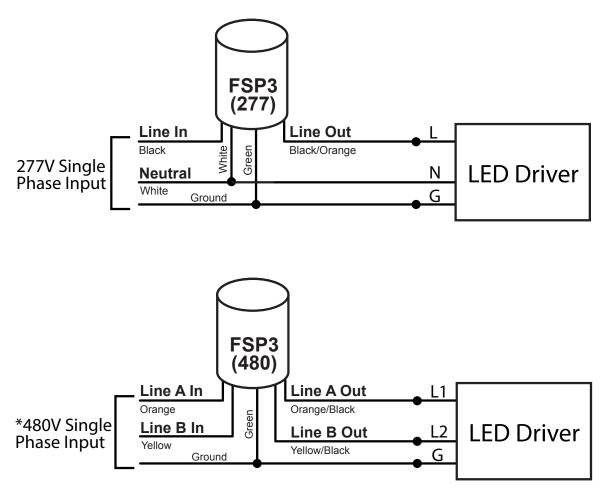
\*A single phase input from 3-phase system uses only 2-phase line connections (A-B, B-C or C-A)
