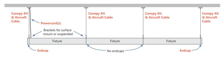
**RED** indicates items that must be ordered as options or accessories. The starter, when suspended, is normally the only fixture in the row with (2) suspension hangers. The rest of the run may be suspended from a single hanger.
