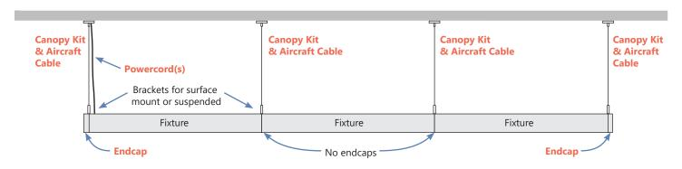
**RED** indicates items that must be ordered as options or accessories. The starter, when suspended, is normally the only fixture in the row with (2) suspension hangers. The rest of the run may be suspended from a single hanger.
