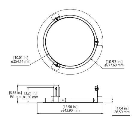
**Compatible Fixtures:** LRC10 **Hole Diameter:** 11.7" – 12.3"
