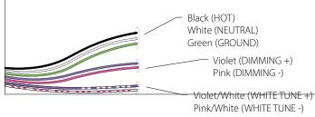
SpectraSync Tunable White luminaires are provided with two 0–10V circuits. The violet and pink circuit is for wiring to any qualified 0–10V controller for dimming. The violet/white and pink/white circuit is for wiring to any qualified 0–10V controller for Tunable White CCT control.
