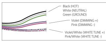
SpectraSync Tunable White luminaires are provided with two 0–10V circuits. The violet and pink circuit is for wiring to any qualified 0–10V controller for dimming. The violet/white and pink/white circuit is for wiring to any qualified 0–10V controller for Tunable White CCT control.
