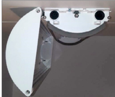
Lens frame will release once the screws have been loosened. The tamper resistant hardware is captured in the lens frame.
