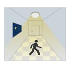
With insufficient daylight, when motion is detected, light turns ON.
