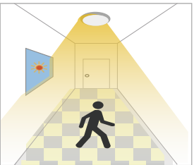
When motion is detected, the sensor will switch on the light to 100% brightness
