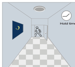
After the last detection and the present hold time is elapsed, light turns OFF.
