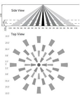
PIR sensor coverage tested as per NEMA WD7-2011
