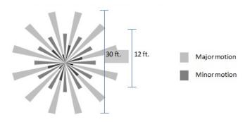
PIR Sensor coverage tested as defined in NEMA WD7-2011
