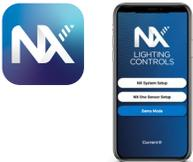
The NX Lighting Controls App is a free to use mobile application for programming both an NX Lighting Controls System or Standalone Bluetooth Sensors. The mobile app allows you to configure devices, discover and setup wireless enabled luminaires and program your NX system settings.
