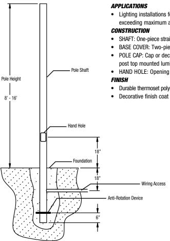
Lighting installations for side and top mounting of luminaires with effective projected area (EPA) not
