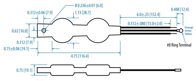
Leads: 6", stripped 0.51" Weight: 0.1 lbs/45g Gauge: 14 AWG
