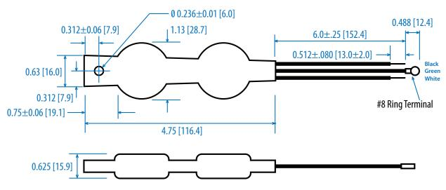
Leads: 6", stripped 0.51" Weight: 0.1 lbs/45g Gauge: 14 AWG
