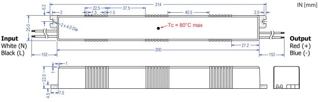
WIRE SPECS: Input Leads: 18 AWG, rated 600 V, 105C, min. Output Leads: 18 AWG, rated 300 V, 105C, min. All wires are stranded with solder dipped ends.
