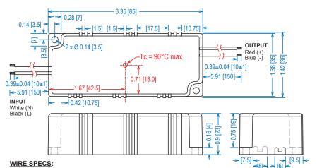
Input Leads: 18 AWG, rated 600 V, 105C, min. Output Leads: 18 AWG, rated 300 V, 105C, min. All wires are stranded with solder dipped ends.
