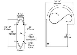
WMA37 Note: Back plate is welded to the arm.
