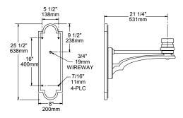
WMA55 Note: Back plate is welded to the arm.
