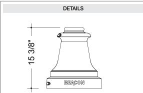
**Note:** Flagler B is a two piece, cast aluminum, decorative clamshell base. Field Installable.
