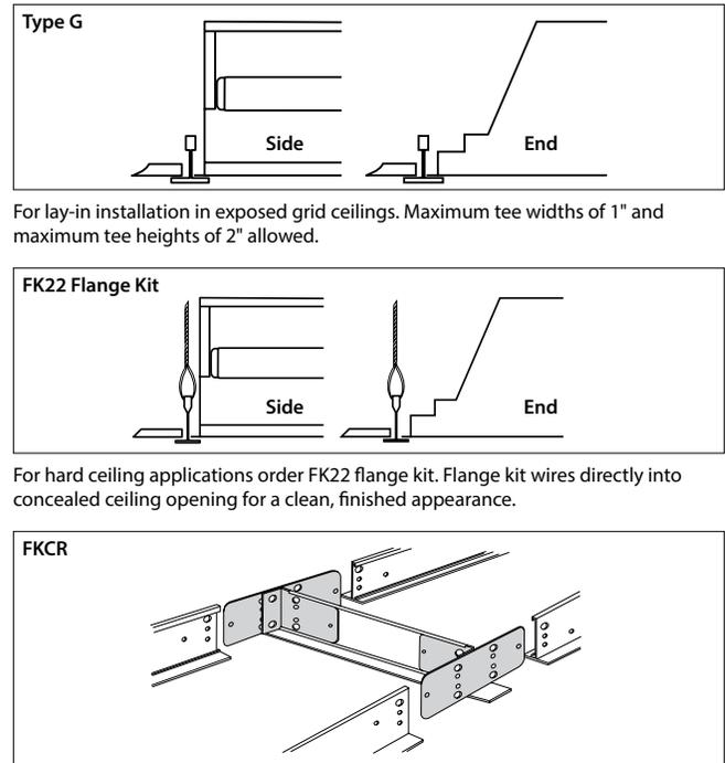
For flanged fixtures in row configurations, the FKCR adapter bracket kit is required in addition to the FK22 kit. Order one less FKCR than the total number of fixtures in row. (Example: Row of two, order (2) FK22 & (1) FKCR)
