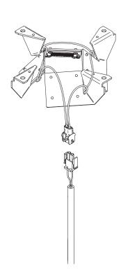
**Electronic Module:** All electrical components are either UL or ETL recognized, mounted on a single plate and factory prewired with quick disconnect plugs. Driver is rated for -40°F starting and has a 0-10V dimming interface for multi-level illumination options.
