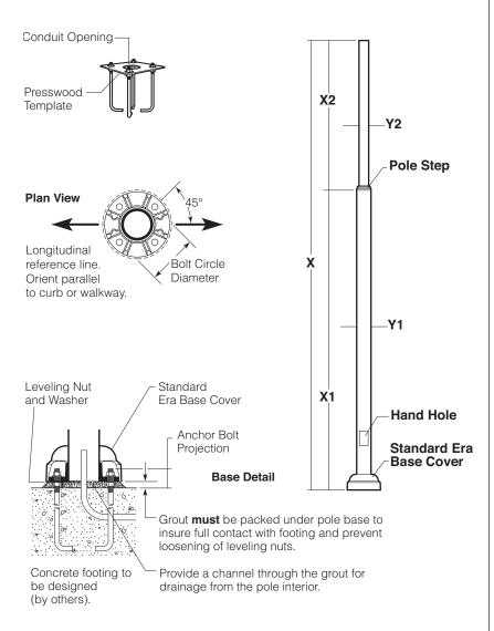
**Pole Construction:** Seamless round extruded aluminum tube of alloy 6061-T6, welded to top and bottom of aluminum base casting of alloy 356.
