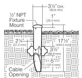
• KLV400 Low Voltage Spear Mount: Die-cast low copper aluminum with 1/2" NPSM fixture mount. Stainless steel set screw locks fixture into mount. Cable slot allows easy fixture mounting before or after installation in ground. Super TGIC powder coat paint over clear anodizing and titanated zirconium conversion coating.
