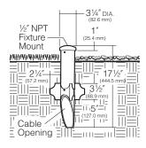
• Low Voltage Spear Mount: Die-cast low copper aluminum with 1/2" NPSM fixture mount. Stainless steel set screw locks fixture into mount. Cable slot allows easy fixture mounting before or after installation in ground. Super TGIC powder coat paint over clear anodizing and titanated zirconium conversion coating.
