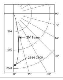
Voltage: 12 Watts: 6.84 Amps: 0.83 Lumens: 470 CBCP: 2344 Beam: 20° CCT: 3000K Efficacy: 69 Lm/W
