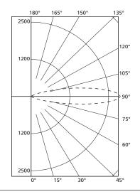
Voltage: 12 Amps: 0.816 Watts: 6.77 Lumens: 460 CBCP: 2264 Beam: 20° CCT: 3000K Efficacy: 68 Lm/W
