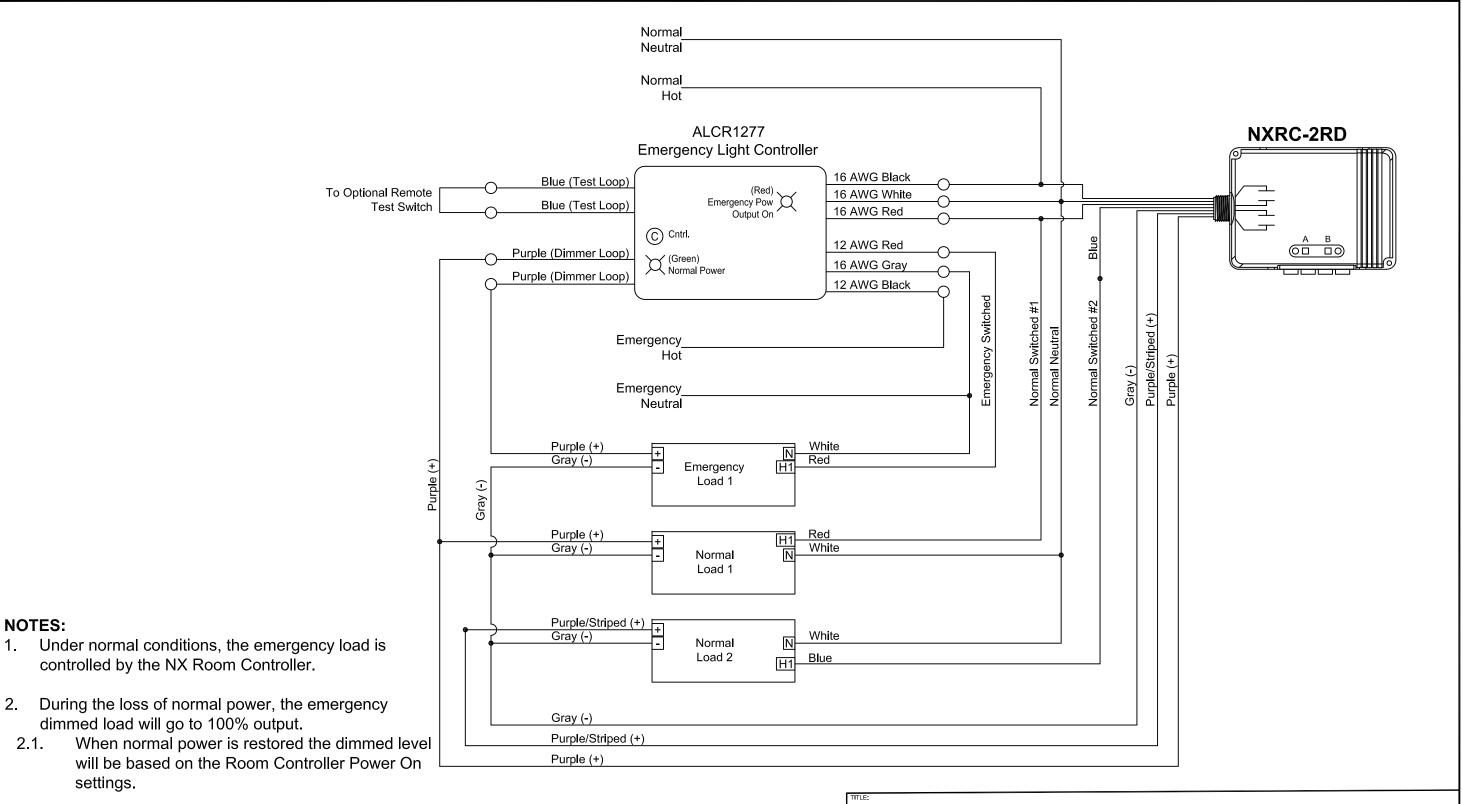
3. During the loss of normal power, emergency dimmed loads will go to 100% output.
