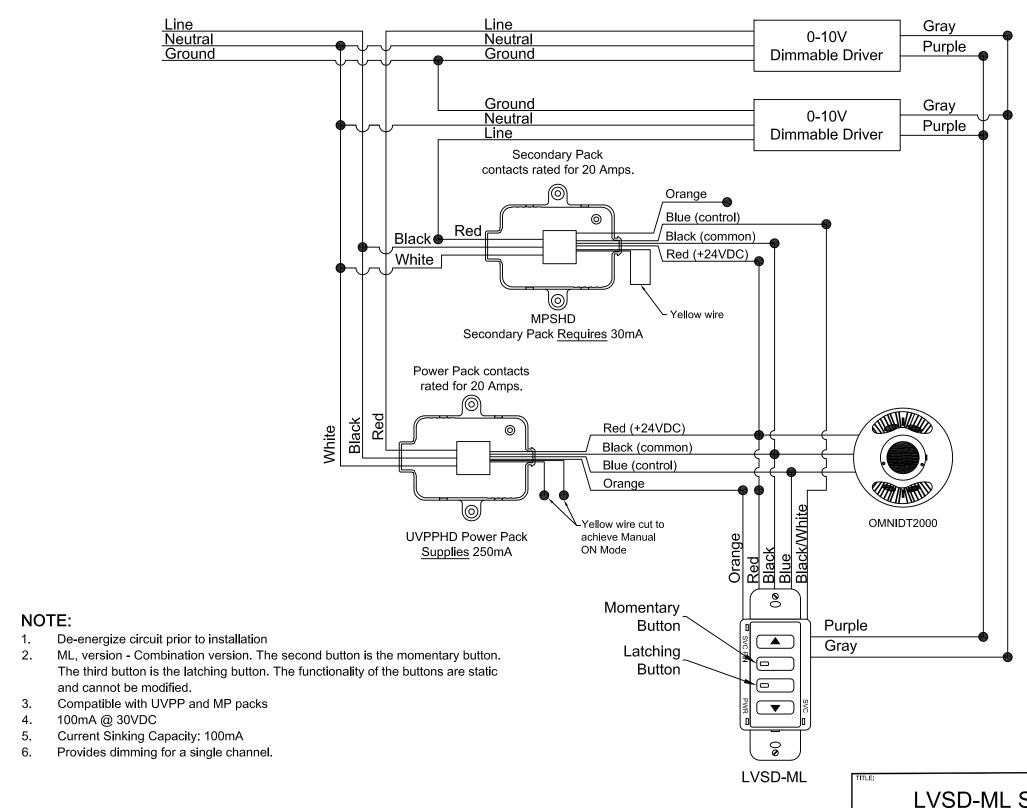
LVSD-ML Switch Station providing 0-10V dimming
