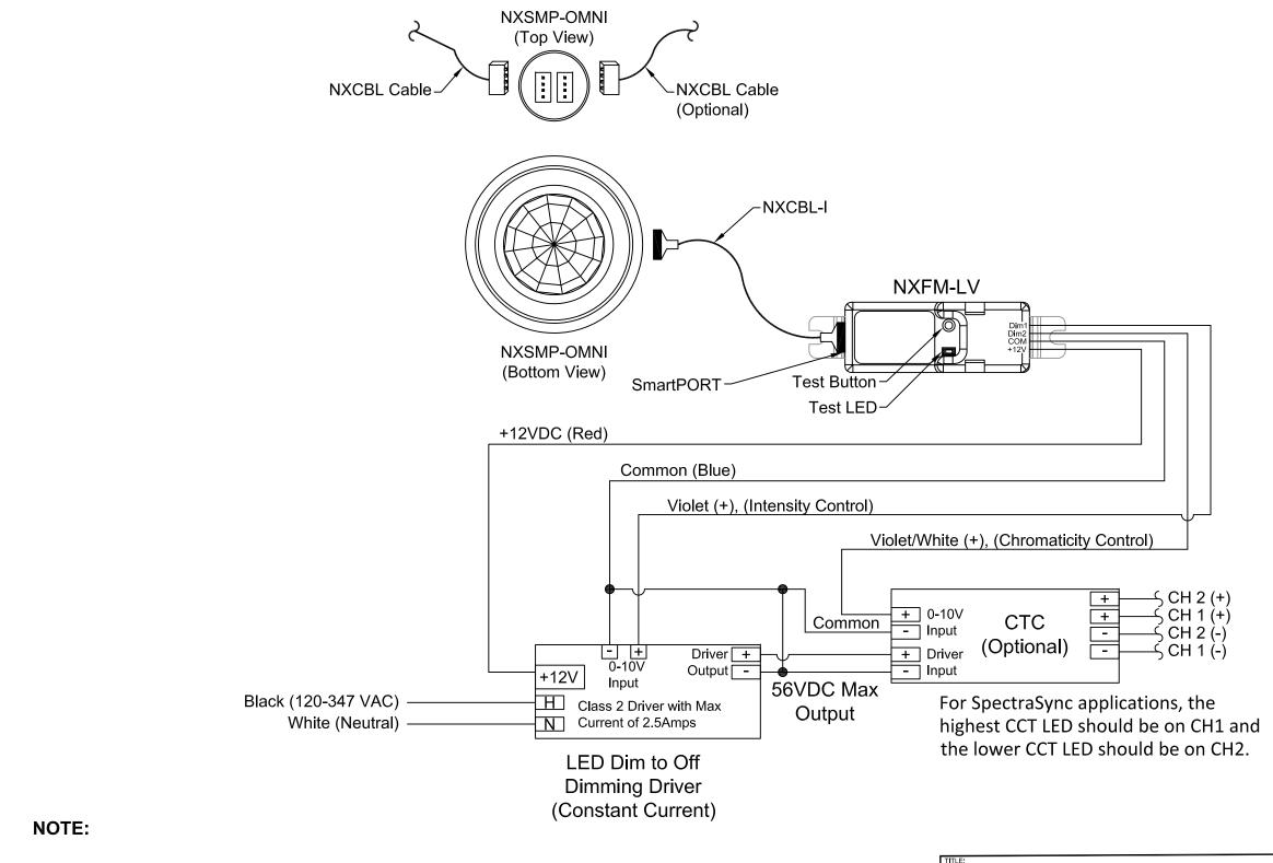
Disconnect power prior to installation.
