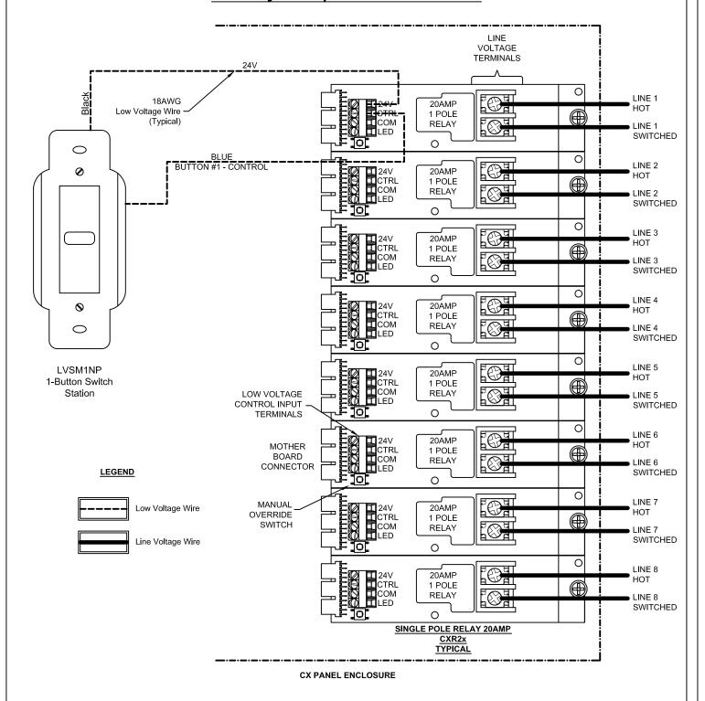
CX Panel with 20 AMP Single Pole Relays Using a 1 Button Low Voltage Switch
