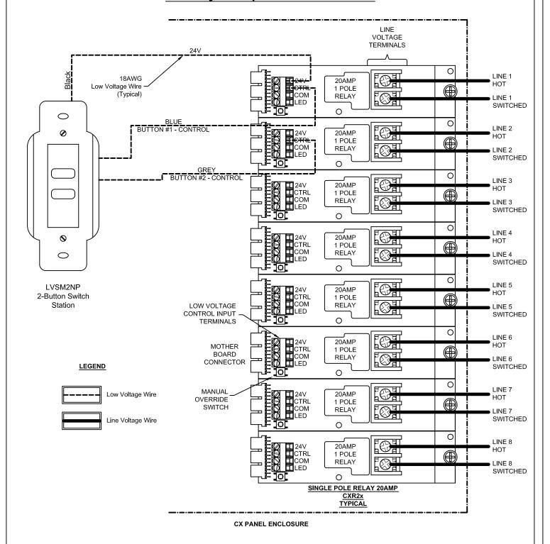
CX Panel with 20 AMP Single Pole Relays Using a 2 Button Low Voltage Switch with No Pilot Lights
